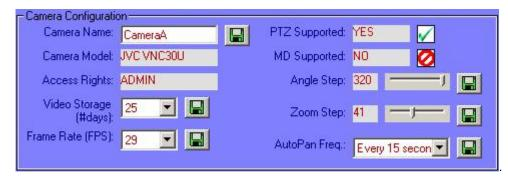
The editable fields are **Camera Name**, **Video Storage (# of days)**, and **Frame Rate (fps)** for all camera models while **Angle Step**, **Zoom Step** and **Auto Pan Frequency** apply only to PTZ type cameras. Once the new information or setting is specified, click on the save button to activate it.
